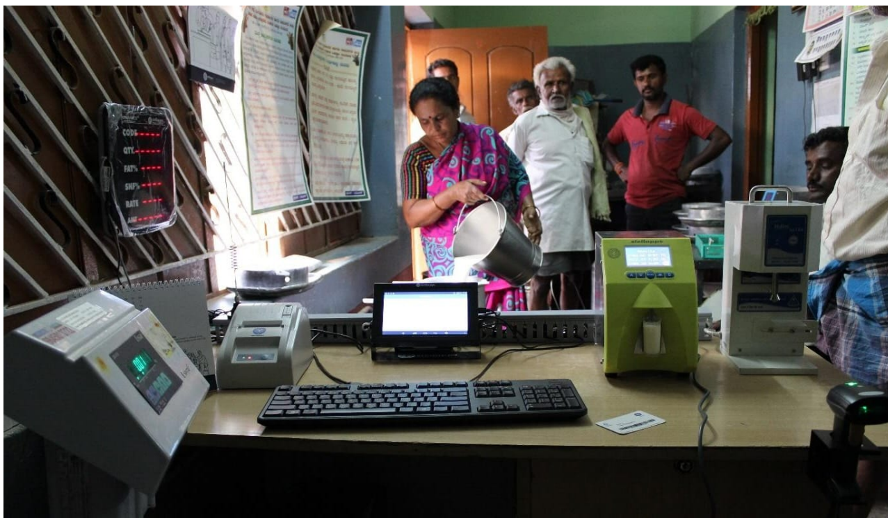
A dairy producer uses an Automatic Milk Collection Unit (AMCU) controlled by an android IoT device. smartAMCU by Stellapps enables IoT-based, real-time acquisition and dissemination of milk procurement data at the collection centres. Photo: Stellapps.
